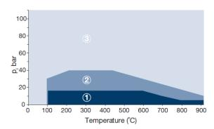
In area 1 the gasket material is suitable using common installation practices subject to chemical compatibility.
