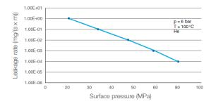
The graph shows the required stress at assembling to seal a certain tightness class. The determination of the graph is based on EN13555 test procedure with Helium at 100°C. The sloping curve indicates the ability of the gasket to increase tightness with raising gasket.
